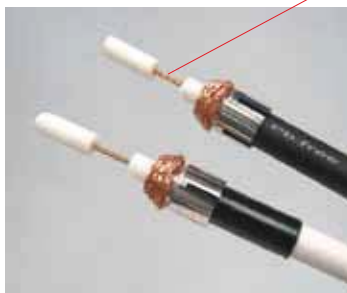
The condition center conductor cut as per the size in drawing at the left after preliminary soldering
